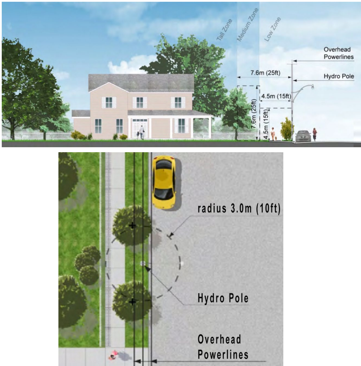
Figure 51: Planting Under or Around Powerlines and Electrical Equipment 11
