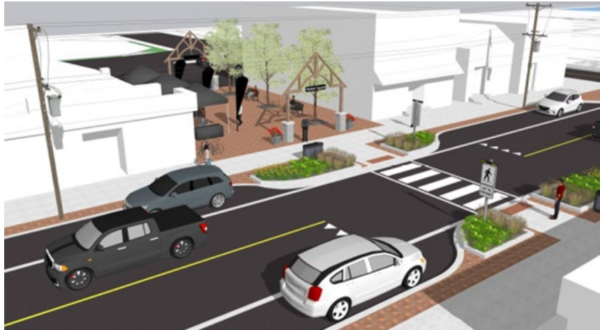
Figure 24: Example of a Pedestrian Bump-out / Curb Extension 6
