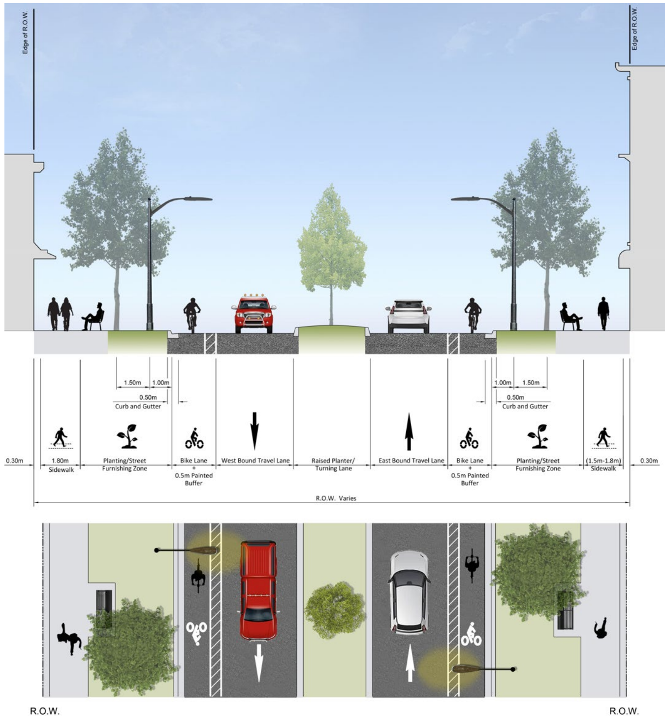
Figure 18: Cross-Section Option for Emerging Main Streets
