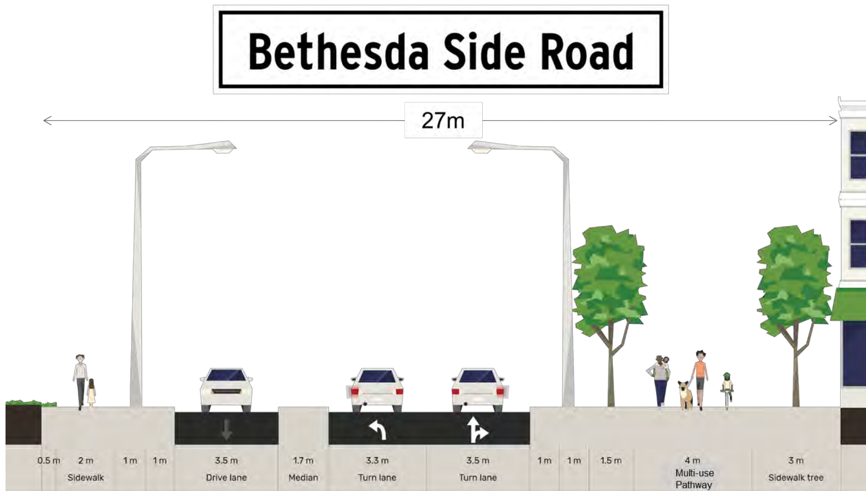
Exhibit 25: Conceptual Typical Cross Section for Bethesda Side Road, Intersection Approach with Left-Turn Lane.
