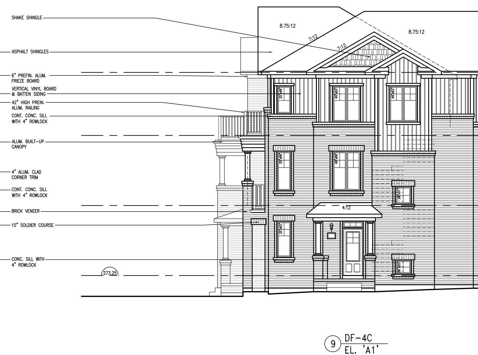
FLANKAGE ELEVATION (EAST)
